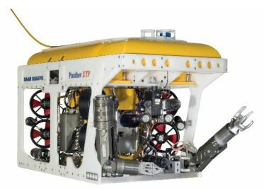
The Seaeye Panther-XT Plus is a high performance Electrically Powered Remote Operated Vehicle (ROV) designed for work and survey tasks in demanding environments.
