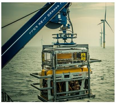
LARS Specifications: Length - 6 meters Width - 2.4 meters Transit height - 3.4 meters Maximum Shipping weight - 22 Tonnes Actual shipping weight - 19 Tonnes Built to - BSEN 12079 Maximum umbilical length - 1600 meters
