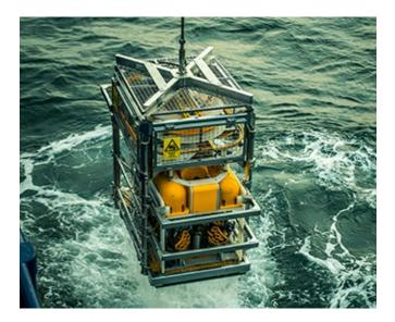
The Type 8 TMS is made from Stainless Steel and designed to be operated in harsh environments. The TMS is used primarily to deploy the Panther safely to the operational depth where it will be working.
