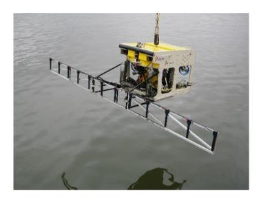
Innovatum SMARTSEARCH is a underwater survey system providing highly detailed magnetic mapping both in marine and land environments. SMARTSEARCH consists of an array of magnetic gradiometers sensors mounted to a frame, which can mounted on an ROV, or towed sled.
